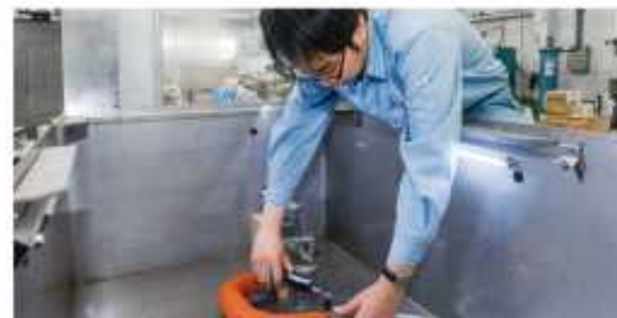
ホース耐圧試験(自作試験装置) Hose pressure resistance testing (Self-made testing device)
